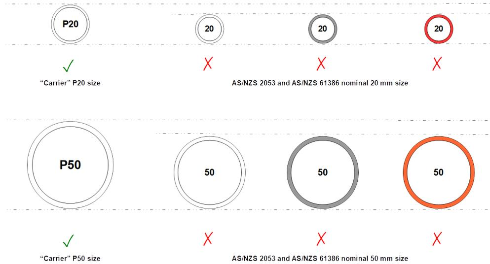
Note: The conduit sizes defined in this Guideline derive from AS/NZS 1477. These sizes are used by telecommunications carriers. Refer to the Definitions section for dimensions of these P20, P50 and P100 "carrier" conduits.
